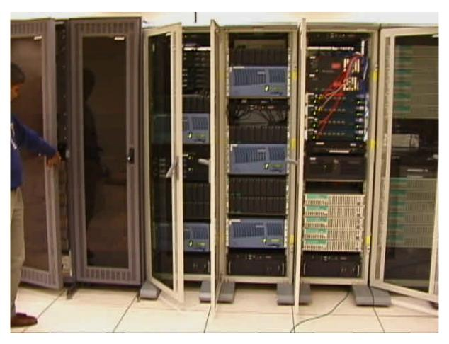
The system shown above is for a high performance web service. It consists of AEI's multi-processor servers running FreeBSD/Unix and Linux, Sun Microsystems servers with Solaris 8/Unix operating system, and networking hardware including firewalls, intrusion-detection, routers, switches, and hubs from Cisco Systems. Network and server load balancers are from Alteon (now Nortel Networks). All networks are 1000FX, and some are 100TX Ethernet. A total of 11 networks are in use.
